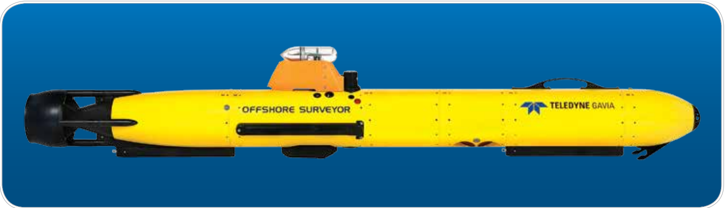
FLS X Series Sonar and Multibeam Profiler Sonar on AUV
